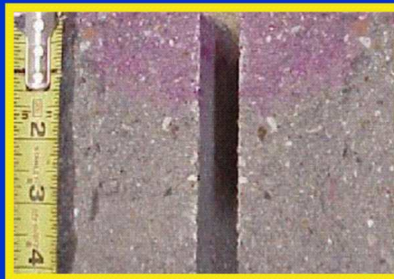
SEAL-A-CRETE™ Typical penetration in 32mpa concrete (with fluorescent dye added)
